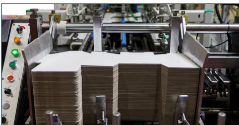
Severe wear caused by abrasive paper products can be eliminated on parts such as guides and fingers of packaging machinery.
