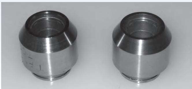
Crimping tool before and after coating with Magnagold.
