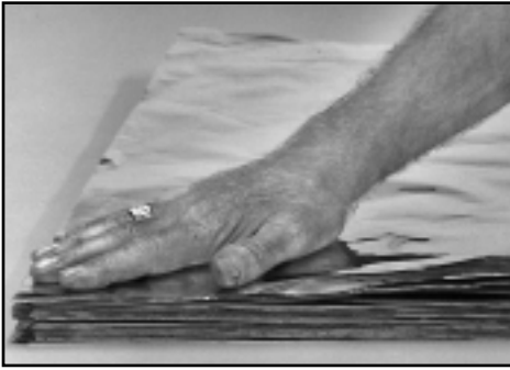
(Left) Lining up closed stack of Scheidl Manufacturing epoxy/glass plies on TUFRAM® coated aluminum platens. Beneath each platen are plies of the next stack. Shiny surface is the next platen. (Right) Assembled stack in the press. Cure cycle: from room temperature to 350°F, remaining at that temperature under 6,000 lbs. psi for 90 minutes. It is then cooled. Fluctuating cycle temperature range creates problems for aluminum platens and molds.
