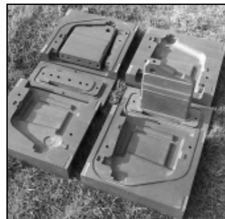
This intricate mold for plastics, used by an electronics manufacturer, was treated with a TUFAM® coating for quick release.
