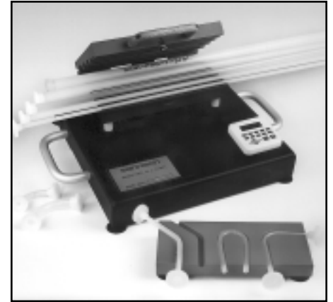
Sani-Tech's tube bending system consists of two primary components: the Sani-Pro Bender that quickly and evenly heats the sanitary tubing, and the Sani-Form, which allows 45°, 90°, and 180° bends to be formed. Keys to consistent bending are Sani-Pro's aluminum molds, which are treated with Magnaplate HCR®.
