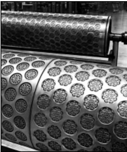
Brass rolls for molding cookies on a high-speed production line at Nabisco were coated with a NEDOX® "synergistic" coating to give longer life to the expensive rotary molds, to prevent dough hang-up by providing mold release, and to make the molds easy to clean.
