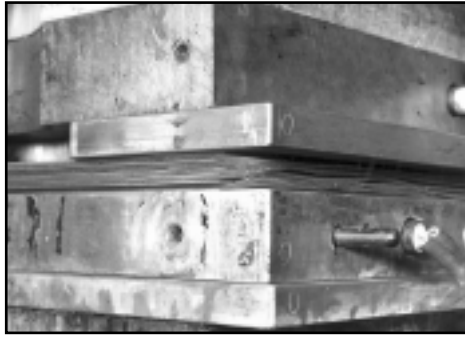
(Left) Lining up closed stack of Scheidl Manufacturing epoxy/glass plies on TUFRAM® coated aluminum platens. Beneath each platen are plies of the next stack. Shiny surface is the next platen. (Right) Assembled stack in the press. Cure cycle: from room temperature to 350°F, remaining at that temperature under 6,000 lbs. psi for 90 minutes. It is then cooled. Fluctuating cycle temperature range creates problems for aluminum platens and molds.
