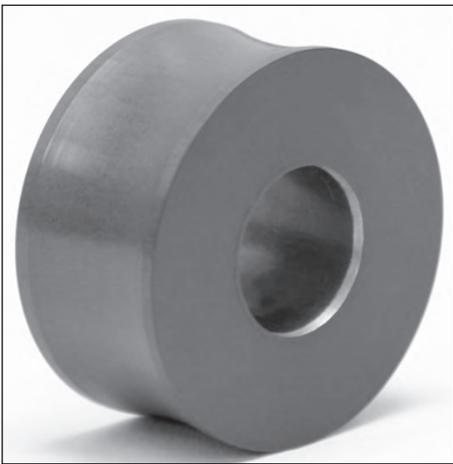
*TUFGRAM provides superior protection in severe abrasive environments. This roller guide is used to manufacture cardboard tubing. TUFGRAM coatings run on Taber abrasion testing units have produced weight loss numbers as low as 0.5 mg per 1000 cycles (Fed Std. #141).*
