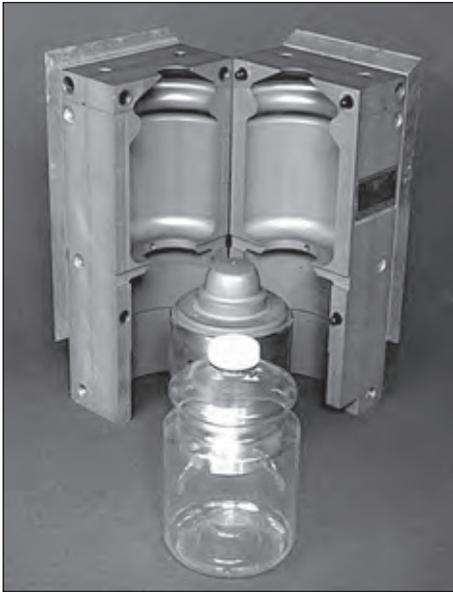
*TUFGRAM on aluminum sections of Johnson Controls' bi-metallic PET bottle molds prevent erosion and galvanic corrosion causing poor release, high reject rates and shortened mold life. Steel sections are treated with Magnaplate's NEDOX®.*
