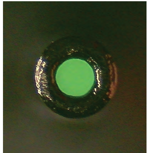
About 0.005 inch of General Magnaplate's Nedox SLK is applied to the inside diameter of the nickel silver nozzle's exit aperture. Once coated, the inside diameter is reduced by about 0.001 inch.
