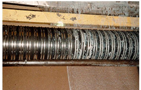
This Sonoco Products Company adhesive metering roll was treated with non-stick, Magnaplate-applied LECTROFLUOR®. Adhesive residues have been significantly minimized. Clean-up between runs is now simple and quick, without the use of harmful chemicals.
