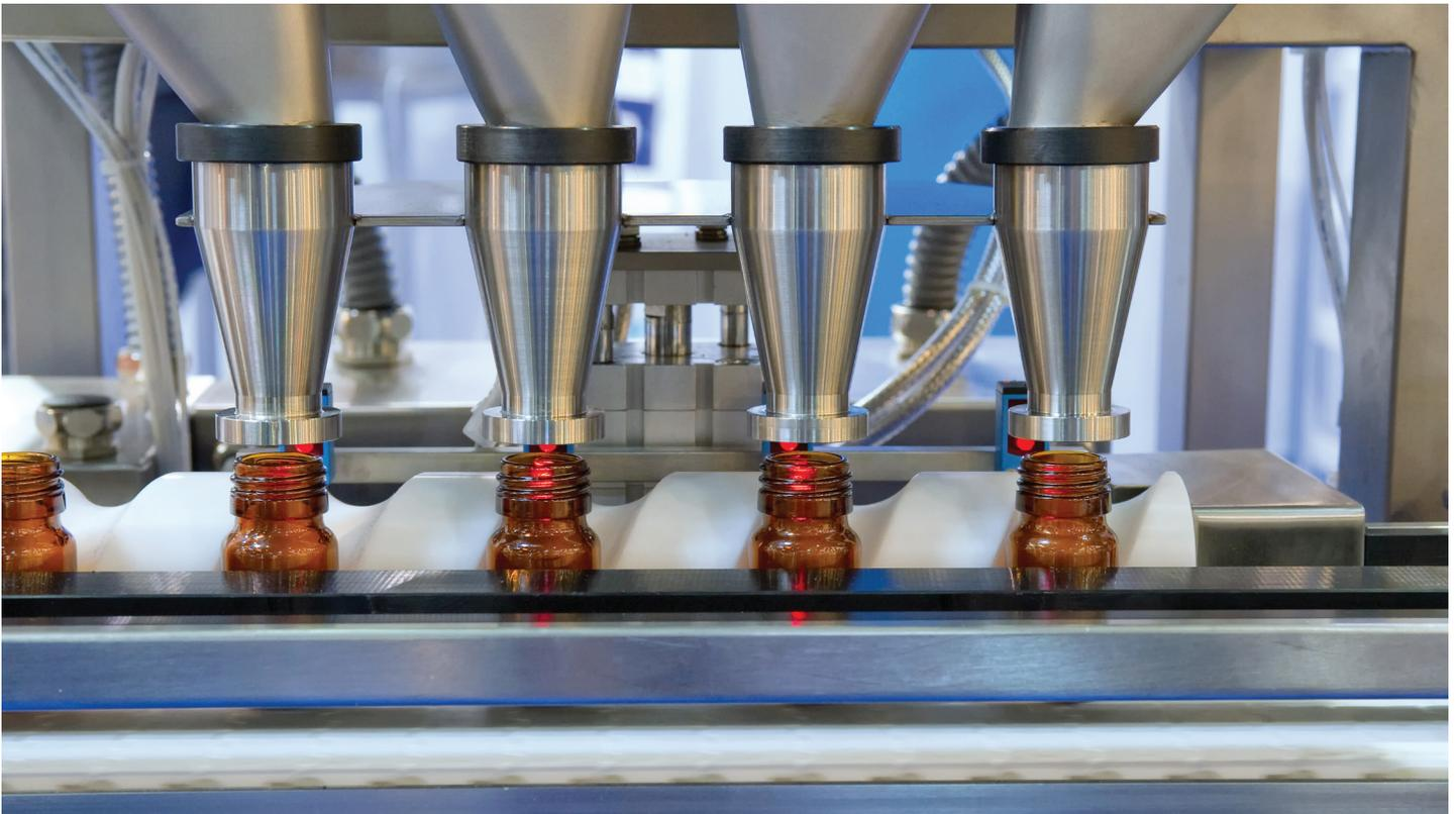
*Applying Magnaplate coatings to pill chutes maximizes throughput and minimizes downtime.*
