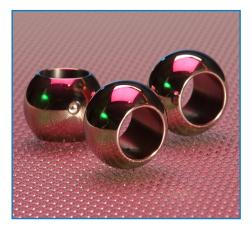
Because of its extremely low coefficient of friction, the MAGNAPLATE HMF coating applied to the SS ball portion of a valve containing a powdered metal seat, eliminates galling that could result in premature wear, leaking and, ultimately, total failure of the valve. In addition, use of the coating permits raising the operating temperature by over +200°F (+93°C), and extends both the active life and shelf life of the valves.
