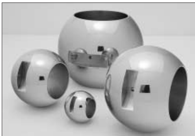
Because of its extremely low coefficient of friction, the MAGNAPLATE HMF coating applied to the SS ball portion of a Worcester Controls valve containing a powdered metal seat, eliminates galling that could result in premature wear, leaking and, ultimately, total failure of the valve. In addition, use of the coating permits raising the operating temperature by over 200°F (93°C), and extends both the active life and shelf life of the valves by 50%.
