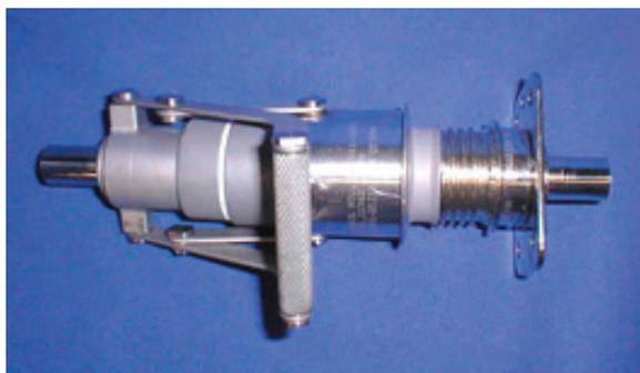
*Quick Disconnect Couplings (QDC) on the International Space Station (ISS) manufactured by the Parker Stratoflex Unit of Parker Hannifin Corporation are treated with a NEDOX synergistic coating to prevent surface scratches which could lead to leakage of system fluids.*
