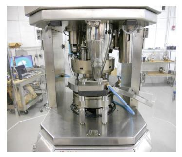
**Tufram For Aluminum.** For the press's aluminum parts, Calvin selected TUFRAM HO. These parts include the feeder, scrapers and deck plates. With a hardness of 40 to 50 Rc and a dry-lubricated surface, TUFRAM gives all these components good release properties relative to the powder. TUFRAM also protects the aluminum parts from wear, corrosion, sticking and galling.
