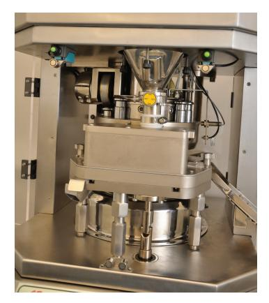
Those product-contact areas include a powder feeder, scrapers and turrets. Left unprotected, all of these components can experience abrasive wear as the machine compresses powdered pharmaceuticals into tablets at pressures up to 20 tons.
