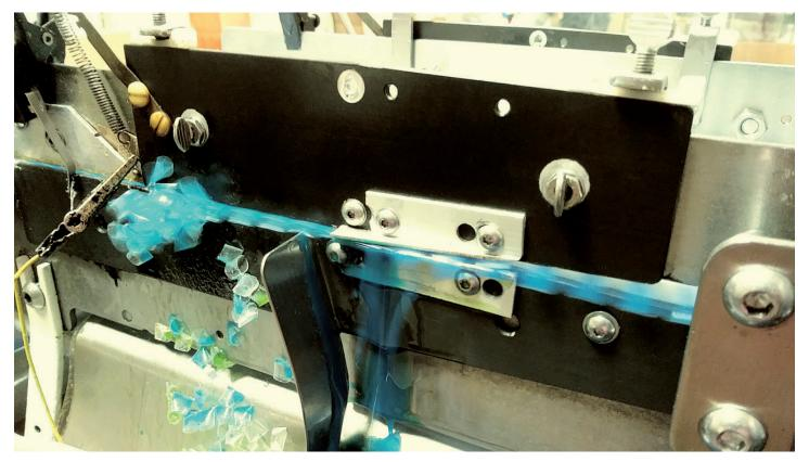
Using patented sealing and cutting blades, the Honeystix machinery cuts and heat-seals 10 honey-filled sticks a second or 13,000 sticks every hour.
