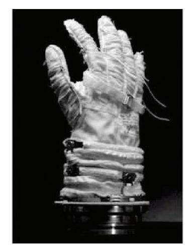
"Magnaplate has a strong track record in space so we approached them about coating the glove ring gimbals," reports Graziosi. "The solution was to coat the parts with Nedox-SF2, a coating which not only provided the required permanent lubricity but also gave us confidence that it would last without being affected by the harsh conditions."
