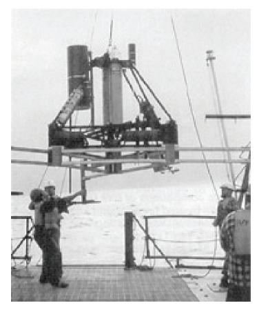
Performance is excellent. Although the tool is continually subjected to pressures up to 15,000 psi and temperatures of  $302^{\circ}F$  (150°C), the tool can stay downhole for up to 30 days.
