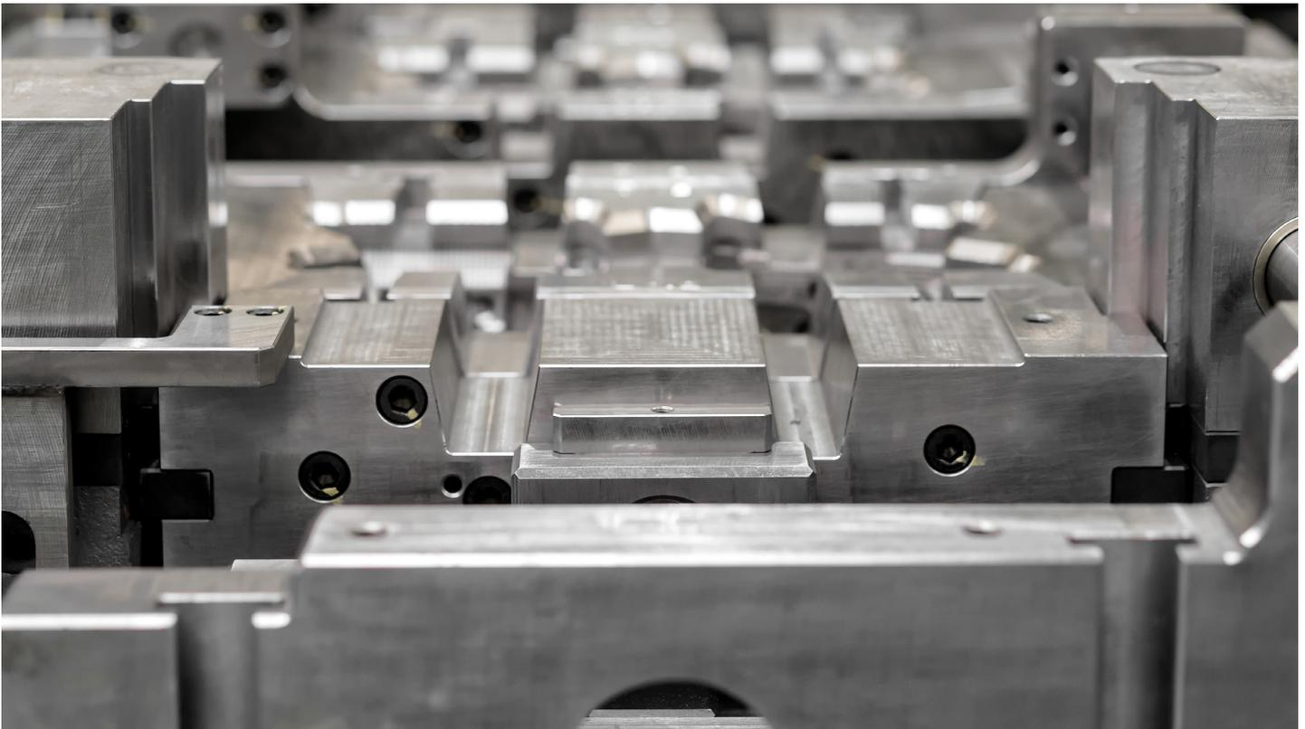
A leading custom profile extruder of plastics attains flawless surface finish quality while doubling die life and increasing productivity by the application of unique, steel-hard coatings to its aluminum extrusion dies.
