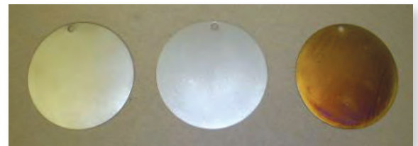
From left, 10K1 coated disc, 10K3 coated disc, electroless nickel-plated disc. Samples treated with 10K1 and 10K3 coatings resist oxidation at temperatures of 1,000° F, while the electroless nickel-plated sample exhibits oxidation and discoloration.
