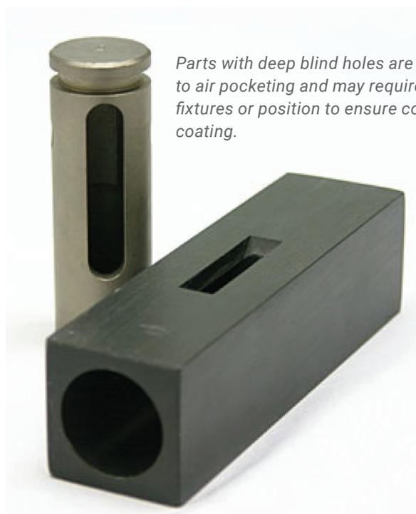
Parts with deep blind holes are subject to air pocketing and may require special fixtures or position to ensure continuous coating.
